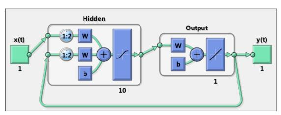
Here the NARX network is used to predict the next output, a timestep ahead of when it will actually appear.
