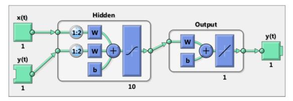
Here the NARX network is simulated in closed loop form.
